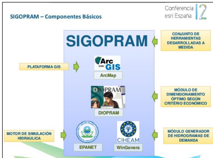
Figura 4.4 – Componentes do SIGOPRAM – (Fortes, 2012)
