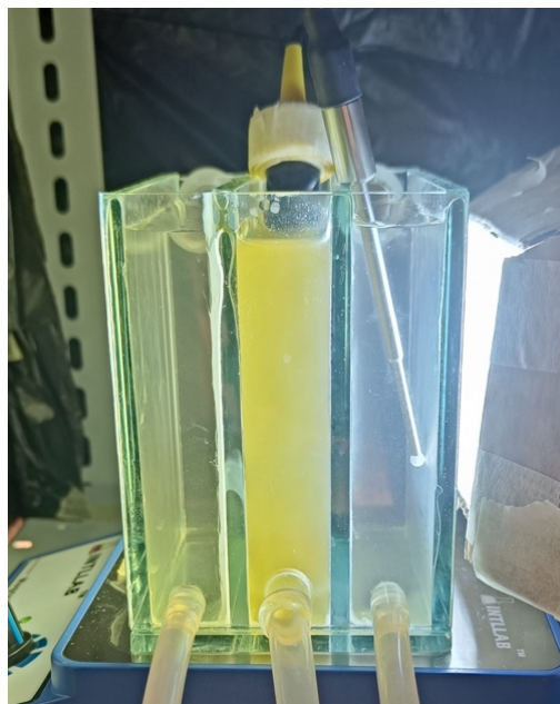
Figure 4 Photosynthetic chamber filled with Phaeodactylum tricornerutum ( 0.2 \text{ g L}^{-1} ) in the middle chamber and filled with distilled water in the adjacent chambers at 22^\circ\text{C} under 500 \mu\text{mol m}^{-2} \text{ s}^{-1} .
