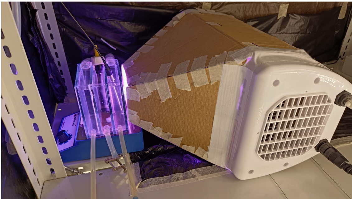
Figure 5. Experimental system with an empty photosynthetic chamber under a wavelength combination ratio of 50% blue (450 nm) and 50% red (620 nm) at 200 \mu\text{mol m}^{-2} \text{s}^{-1} .
