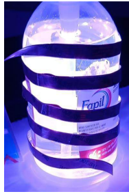
Figure A.4 - 2 AlgaeLum version 0 composed of a flask surrounded by an LED strip in a spiral.
