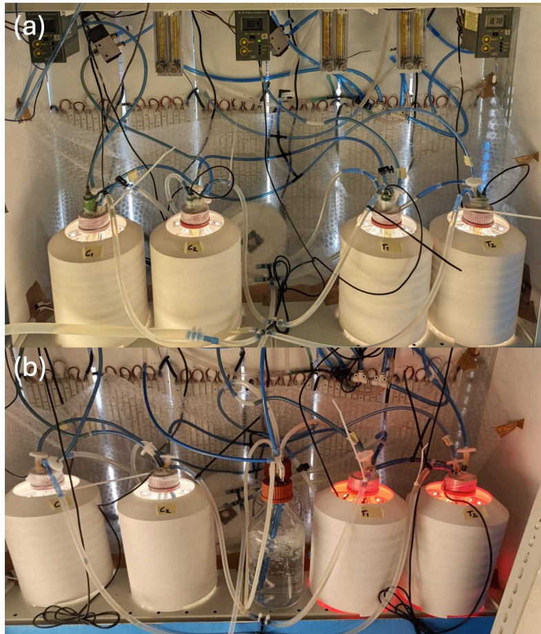
Figure 8 Cultivation setup of the control warm-white and light regime experiment on Phaeodactylum tricoratum . Image (a) shows the setup from 0.2 \text{ g L}^{-1} to 2.0 \text{ g L}^{-1} , using warm white light, 500 \mu\text{mol m}^{-2} \text{ s}^{-1} , and image (b) shows the setup past 2.0 \text{ g L}^{-1} , using 100% red light, 500 \mu\text{mol m}^{-2} \text{ s}^{-1} .
