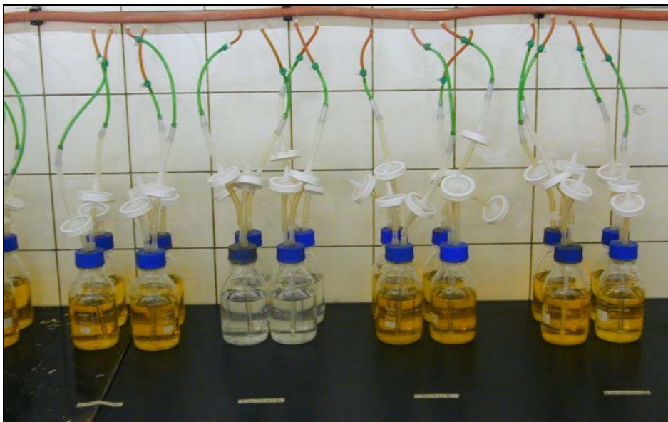
Fig. 4 Experimental set-up showing the bottles, filters and aeration system
