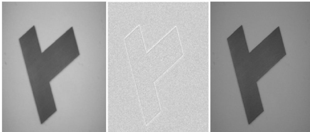
FIGURE 2.4: Edge Enhancement using Unsharp Mask operator[38]
