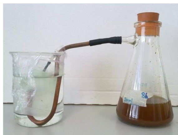
Figure 2 Conical-flask fermenter with gas collector on side-arm.
