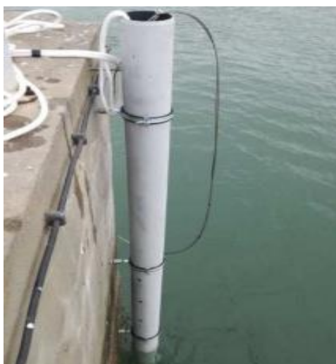
Figure 2.4: PVC tube for the support and protection of the probe (37°00'9.92 N, 7°55'16.28'W).
