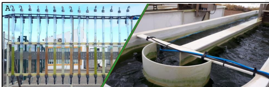
Figure 4.1: Microalgae production systems used to carry out the experimental trials: Tubular bubble column photobioreactors (A) and pilot-scale raceway pond (B)
