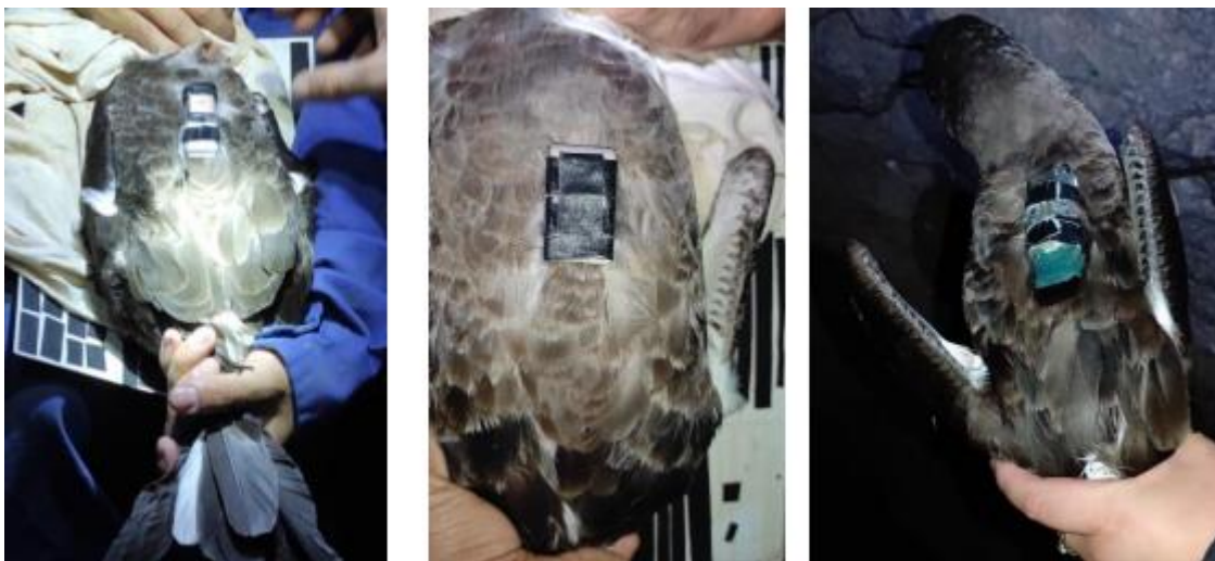
Figure 3.3 Tracking devices deployed on Cory's shearwaters, Calonectris borealis , from left to right: GPS CatLog, GPS Axytrek and GPS XSputnik. Author: Marta Nadal.
