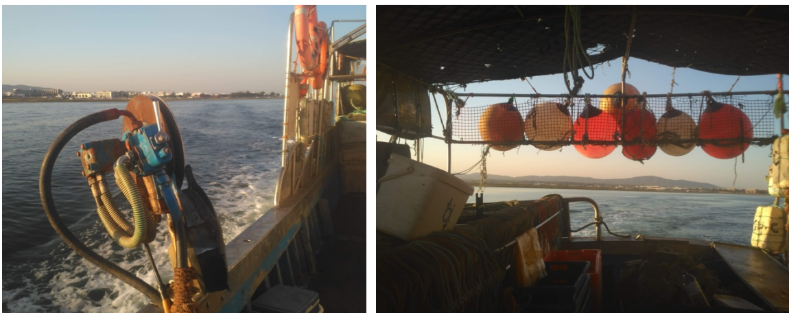
Figure 1.2 - On the left (A) the hydraulic hauler that pull the main line and the traps. On the right (B) the deck of the vessel where the cages are stowed. This area is covered by a structured that do not allow the traps to fall from the boat.
