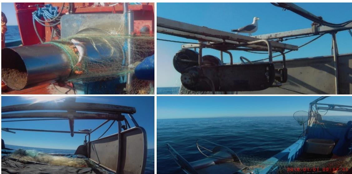
Figure 1.3 - On the left top corner (A) is the hauler system pulling the net. On the top right (B) the sorting system and below, the deck area where the nets are kept after organized.
