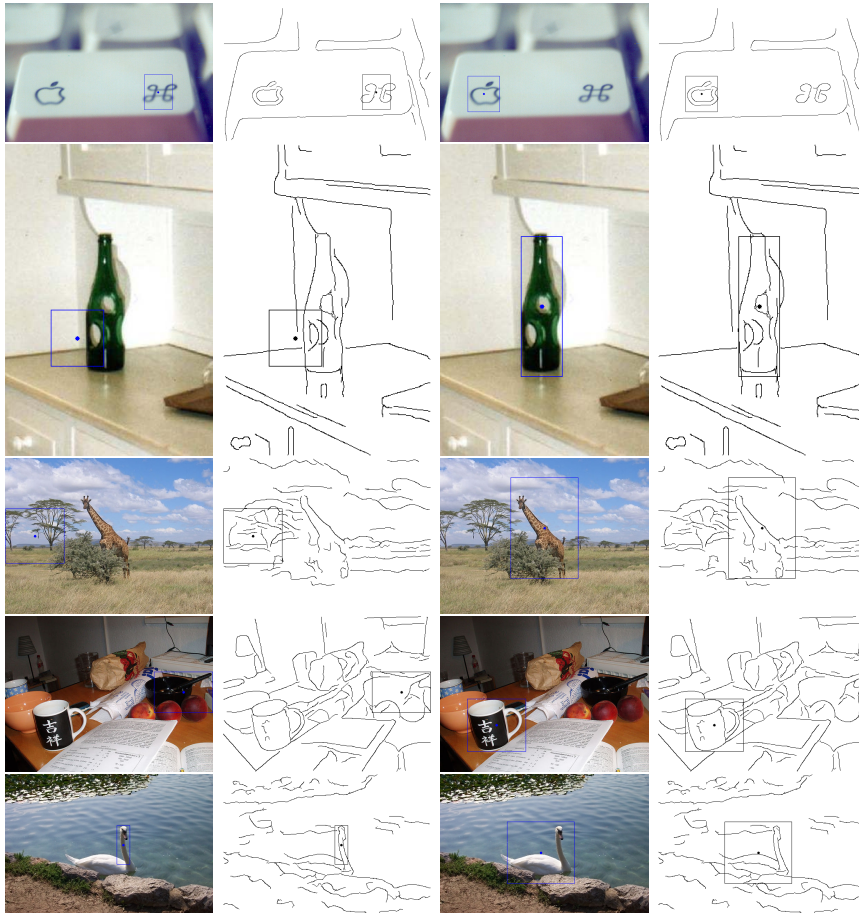
Figure 5.4: Examples of detected objects and their bounding boxes by using the Bayesian discrimination criterion. The black dots are the centres of the boxes. The first and second column show false positive detections. The third and fourth column show true positive detections.
