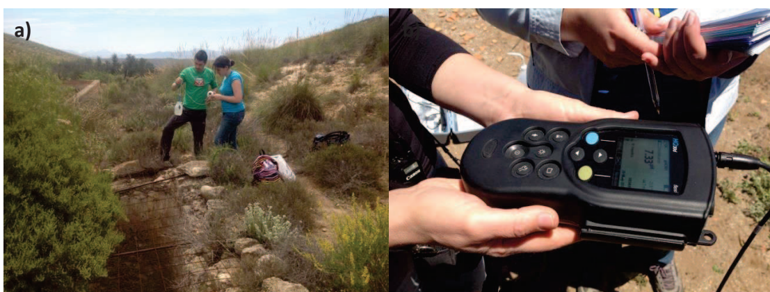
Figure 8. Field work: a) Water sampling b) Measurement of pH, Electrical Conductivity and Temperature.
