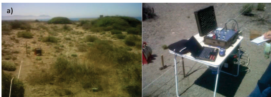
Figure 11. Field work: a) Class A or B electrode and wire coil 500 meters in the field. b) Photography Geotron device used in the field (symmetric Schlumberger)
