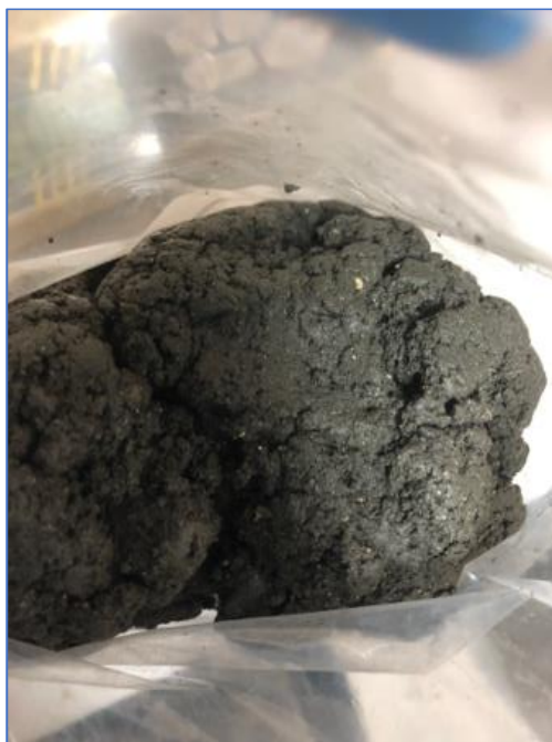
Figure 2.1. Dehydrated sewage sludge obtained from a WWTP in Europe with a granular bioreactor.
