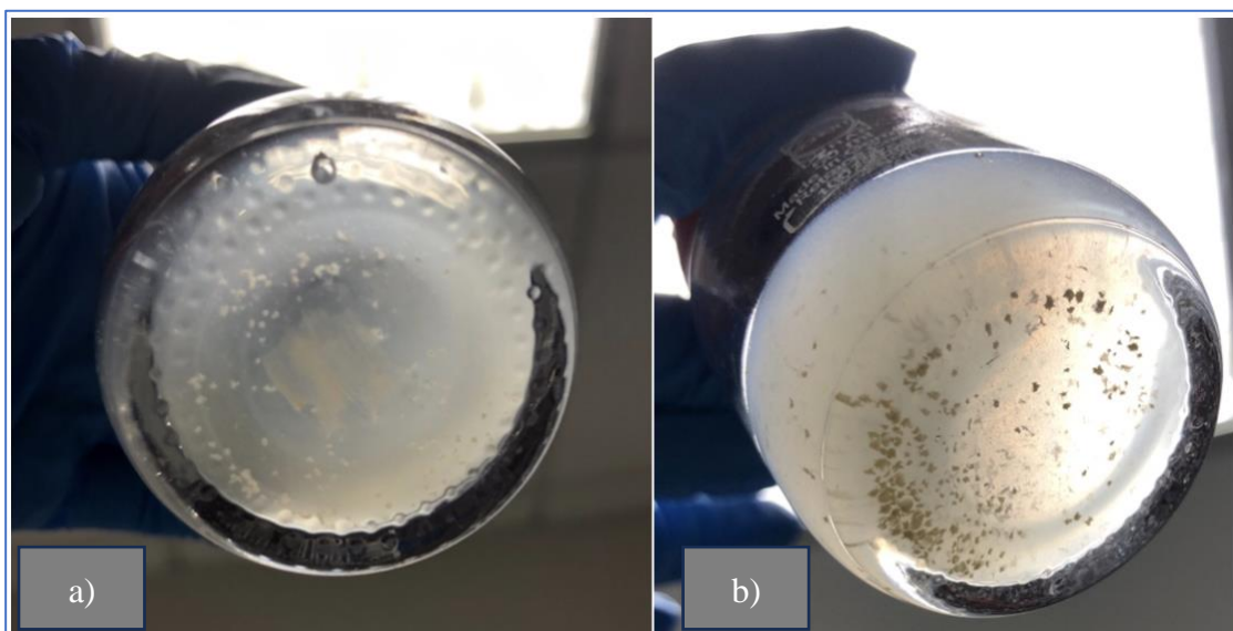
Figure 2.8. Bioaugmented bacteria from genus Bacillus suspended in MSM after 24 (a) hours and after 48 hours (b)
