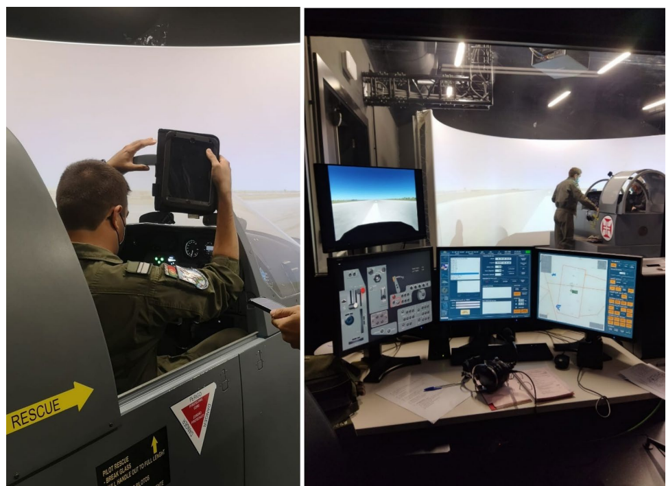
Fig. 2 Left, the inside of the cockpit for the flight simulator Epsilon TB30 and a pilot ready to start the protocol; right, the inside of the control room and the setup device of the flight simulator operator
