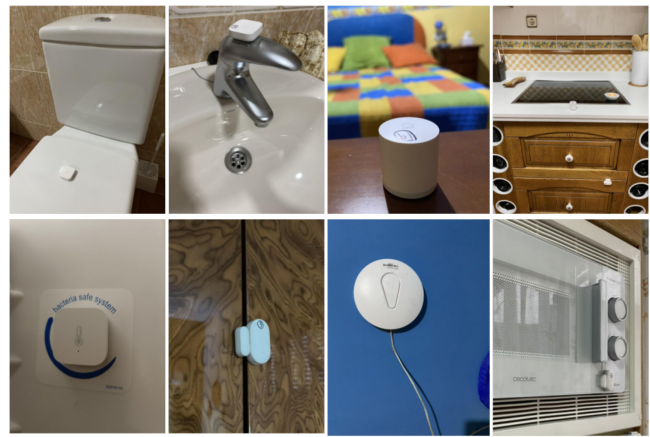
Fig. 9. Deployment of ambient sensors in the real environment, including motion sensors, door/window sensors, vibration sensors, and temperature/humidity sensors. The images demonstrate the unobtrusive placement of the sensors on everyday household items, such as faucets, doors, and appliances, highlighting their minimal invasiveness and seamless integration.
