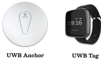
Fig. 2. Overview of UWB devices deployed for indoor location of individuals within the environment. The deployment uses anchors and wearable UWB tags (wristwatches) assigned to each resident.
