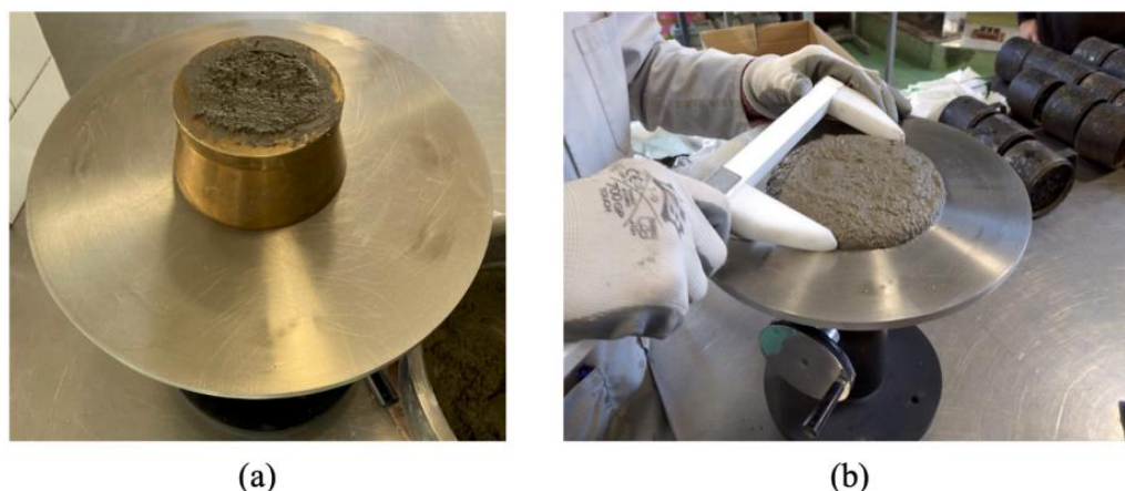
Figure 3. Flow test. Truncated mold (a) and measurement of the diameter of the mortar (b).
