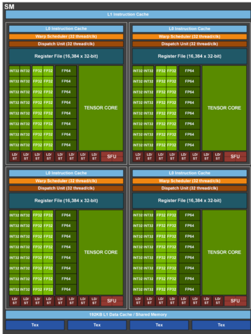
Figure 2.2: A100 GPU Streaming Multiprocessor Detail. (Source: Nvidia)
