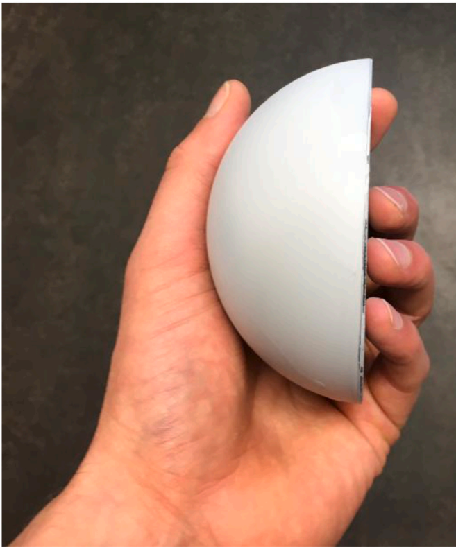
Fig. 2. Near-hemispherical painted glass blank used in the Arbitrary Shape Study. Human hand for scale.
