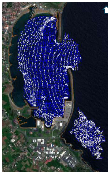
Figure 3.6- Bathymetric survey in 2017 covering the harbour basin and an area in front of the south breakwater (Source: LNEC)
