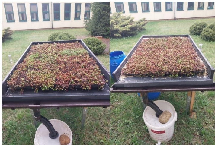
Figure 2.10. EPDM roof with small buckets of Sedum (left) and EPDM roof with small buckets of Sedum and Caxit sorbent material (right).
