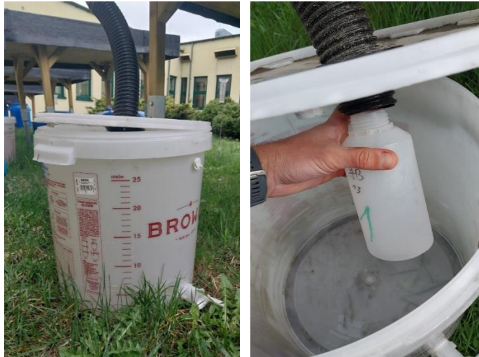
Figure 2.8. Containers used for rainwater collection of experimental roofs.
