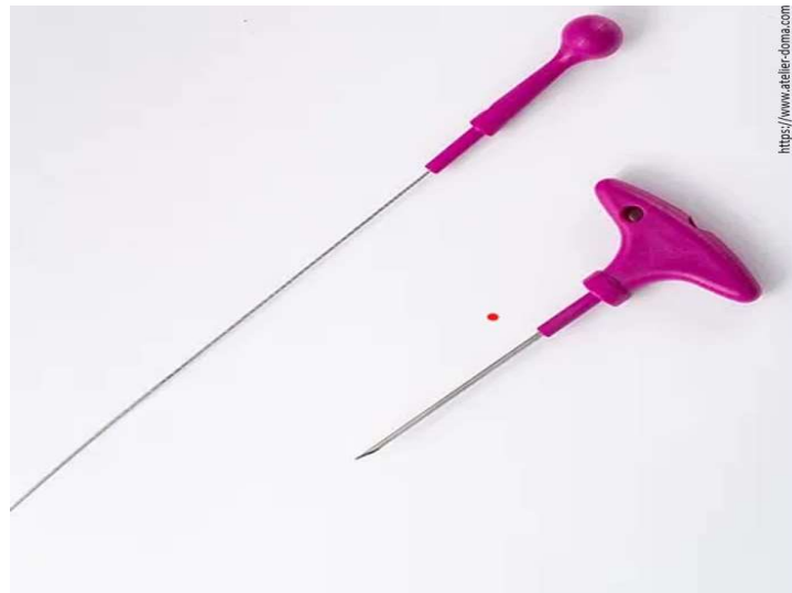
Figure 3.4: Ikejime Tool. Ikejime tool used on the trial (© LumicaDirect.com ). The shorter tool is used for skull penetration and the steel wire for destruction of the spinal cord, through the neural canal.
