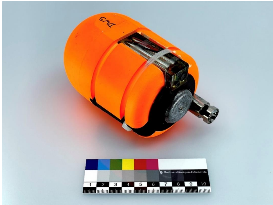
Figure 2.1. Pop- off MultiSensor (MultiS) archival tag. (Photo by: Movement Ecology - MOVE, CIBIO).
