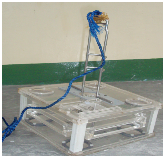
Figure 20. The light trap used for fish larvae recruitment in this study.
