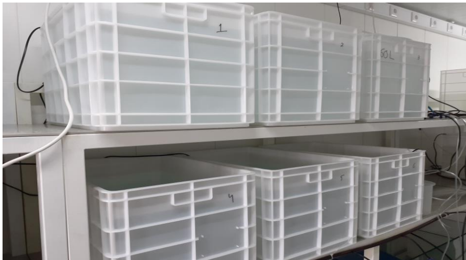
Figure 2.1 Trial tanks set-up. Three control tanks on the top, and three infection tanks on the bottom. Trial worked on a closed system, with only aeration being provided. Water was kept at 23°C, and half of the volume was renewed 24h post infection.
