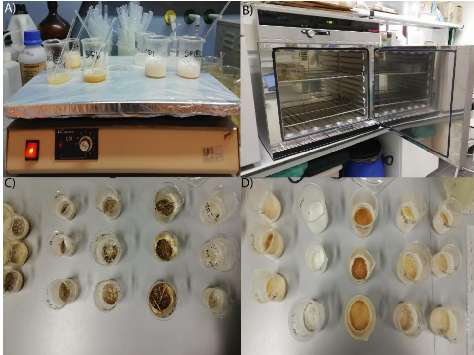
Figure 10: Laboratory work for the DR estimation, (A) reaction of the OM with the H_2O_2 ; (B) samples in the oven; (C) samples before the destruction of the OM; (D) samples after the destruction of the OM
