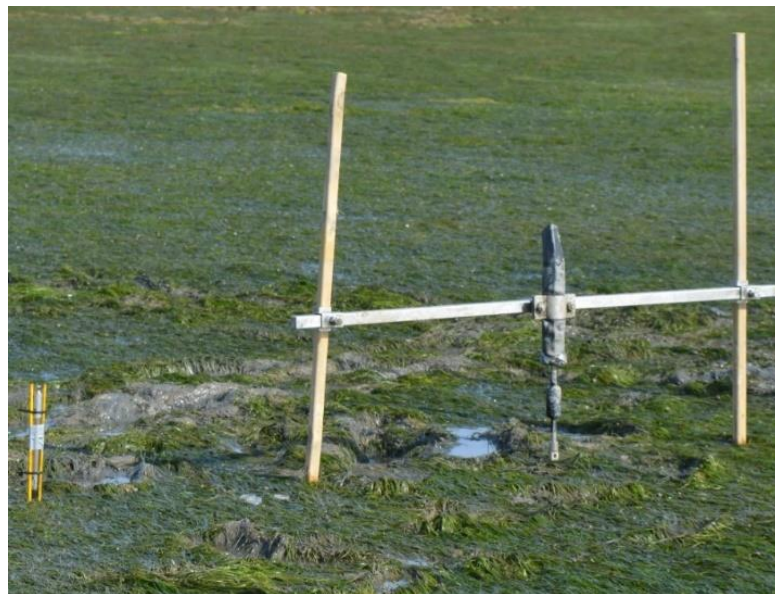
Figure 7: Photo of the EMCM in the field (mounted on a support structure; EMCM is in the middle of the horizontal steel bar), and PT (next to the structure, on the left) at the TF2 station during the 28th of February campaign
