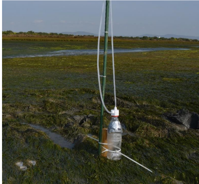
Figure 8: Sediment traps (on the bottom left corner) and siphon sampler (in the middle) at TF1 on the 28th of February
