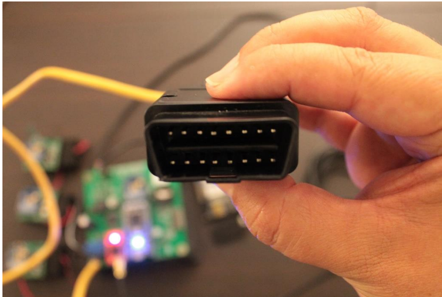
Figura 37 - Pormenor Conector OBD-II
