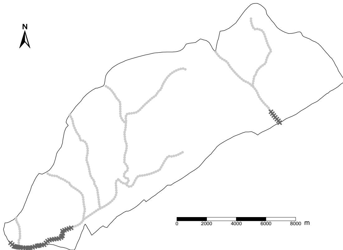
Figure 20 – Watercourses of creeks (light grey lines) and imposed potentials (dark grey crosses) at areas where there is known evidence of occurrence of discharge episodes.
