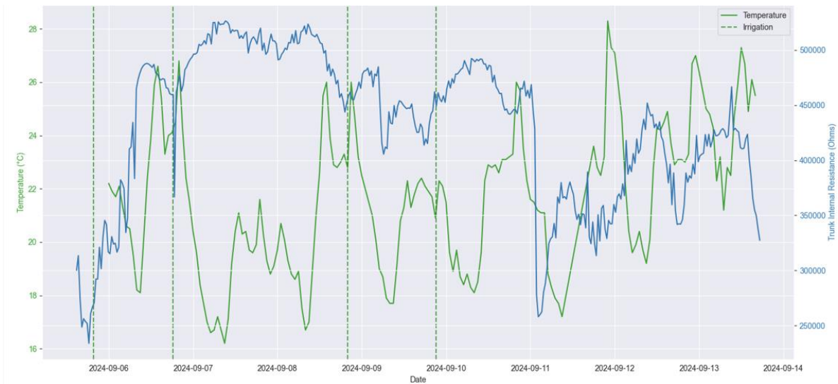
Figure 4.1. Trunk internal resistance (lemon tree) & temperature
