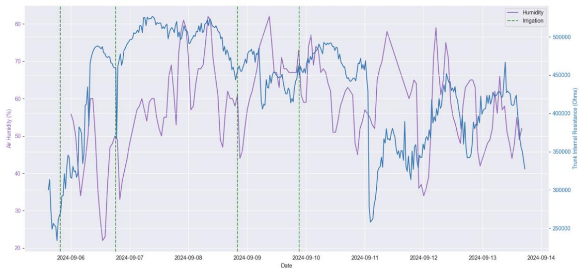
Figure 4.3. Trunk internal resistance (lemon tree) & air humidity
