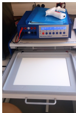
Figure 2.3. Serva HPE Blue Horizon flatbed electrophoresis system with the plate, where the gels are placed, and the power supply
