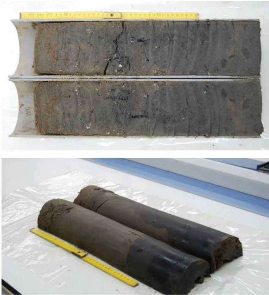
Figure 6.1- Measurements and separation of the collected core before sampling
