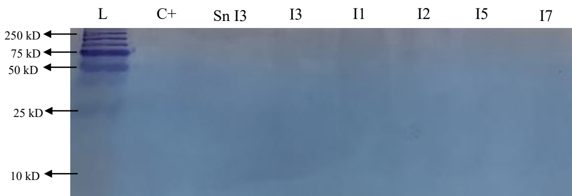
Figure 4.23 Zymography was done using SDS-PAGE stained with methylene blue to identify the fraction responsible for killer activity by a colourless area. No colourless bands are observed.
