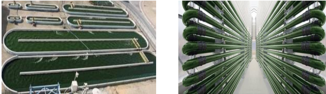
Fig.1.4. Photo of open system - raceway (left) and closed system-tubular photobioreactor (right)
