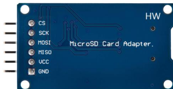
Figura 31 MicroSD Adapter Pinout
