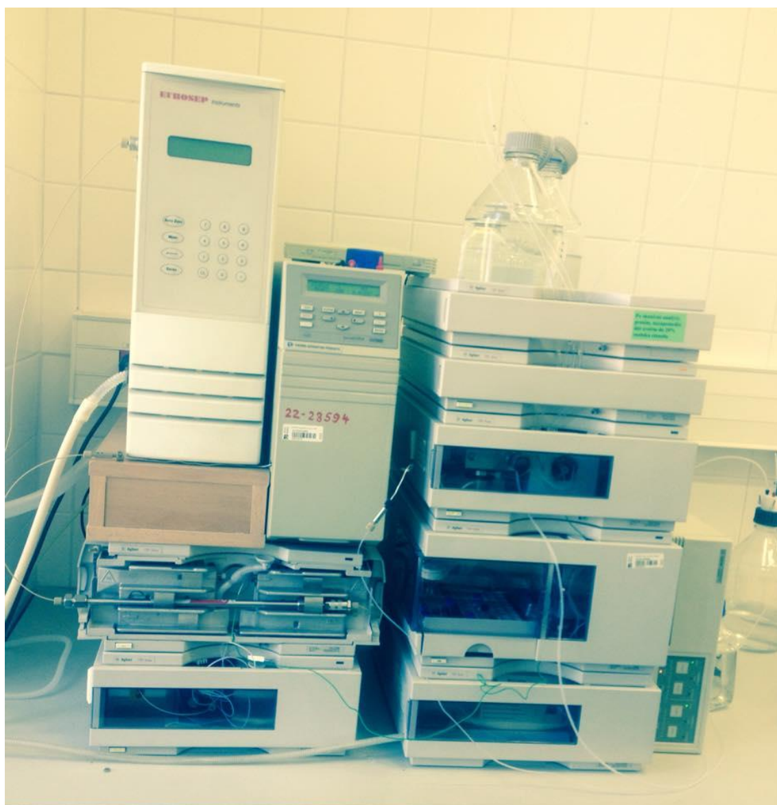
Figura A.1. Equipamento de HPLC Agilent 1100 Series (Agilent Technologies, Santa Clara, CA, USA)
