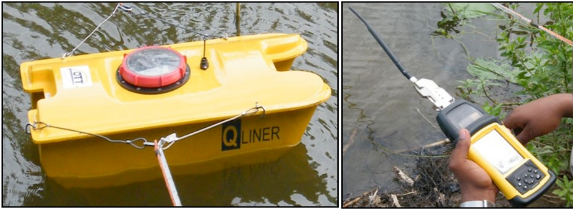
Figure 2: OTT Qliner, A system for mobile discharge measurement in rivers
