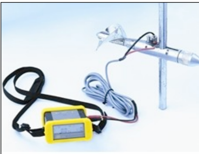
Figure 4: OTT Signal counter (Source: http://www.ott.com )
