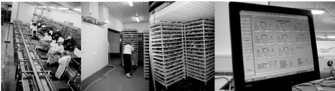
Figure 1.11 - Modern computer-controlled drying facility for cod heads: heads processing, racks transport, racks in the primary drying chamber and control board (Kristbergsson and Arason, 2007).
