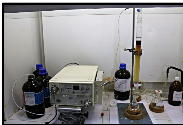
Figure 7.4. Column chromatography separation apparatus.
