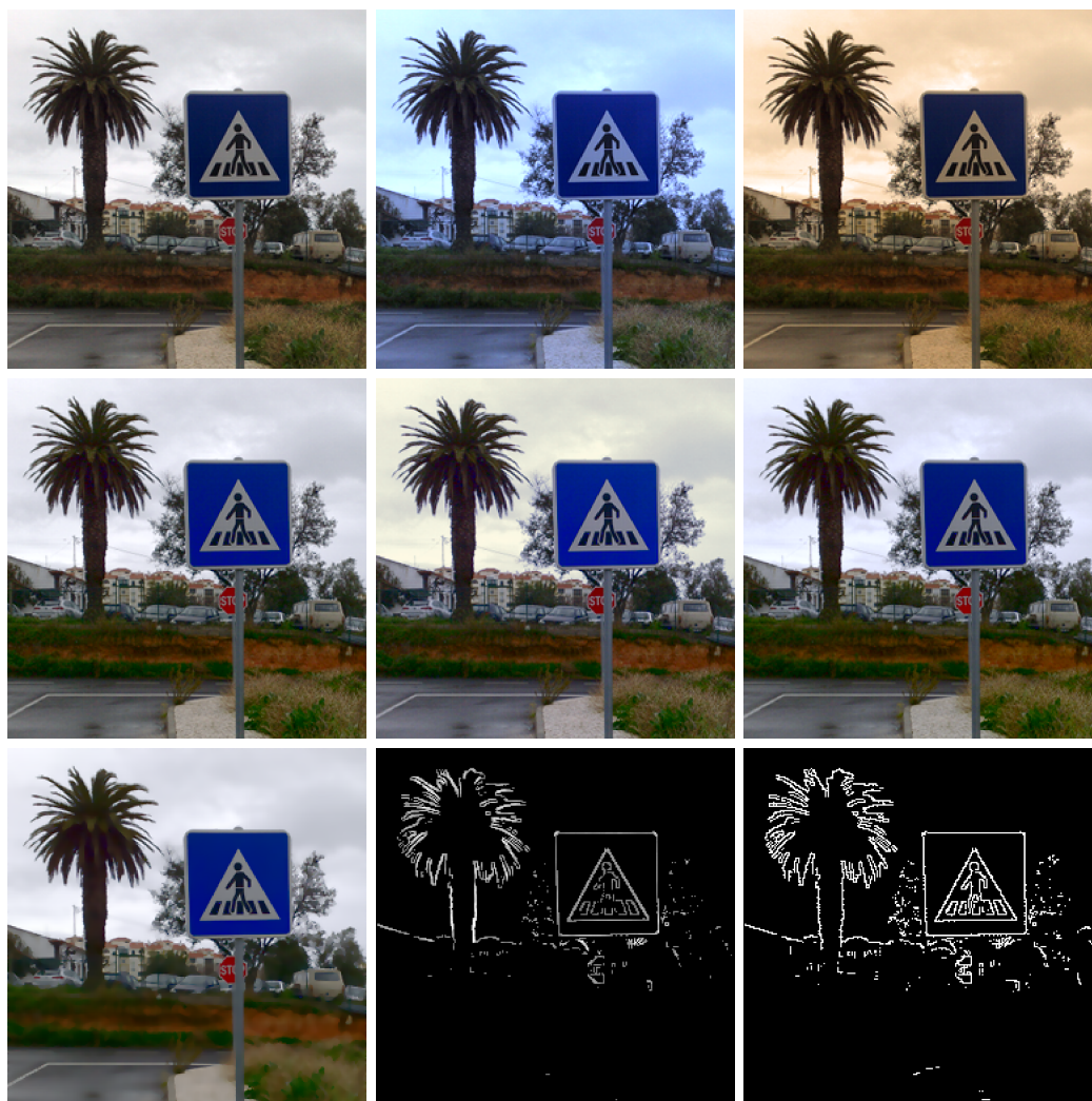
Figure 2.3: Top and middle : colour illuminant and geometry normalisation; input images ( top ) and respective results ( middle ). Bottom, left to right : adaptive colour-region filtering, border saliency by colour conspicuity, and non-maximum suppression.
