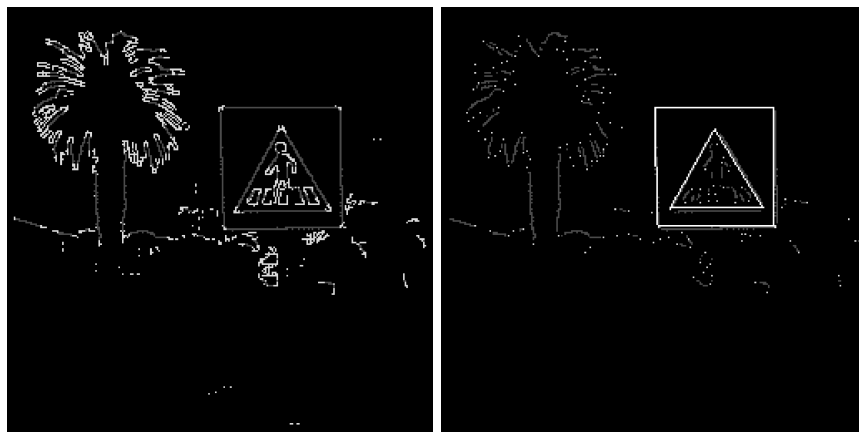
Figure 2.5: Left : cell layer \Xi^{\text{BCo}} for the illustration image before corner condensing. Right : after corner condensing and shape retrieval.
