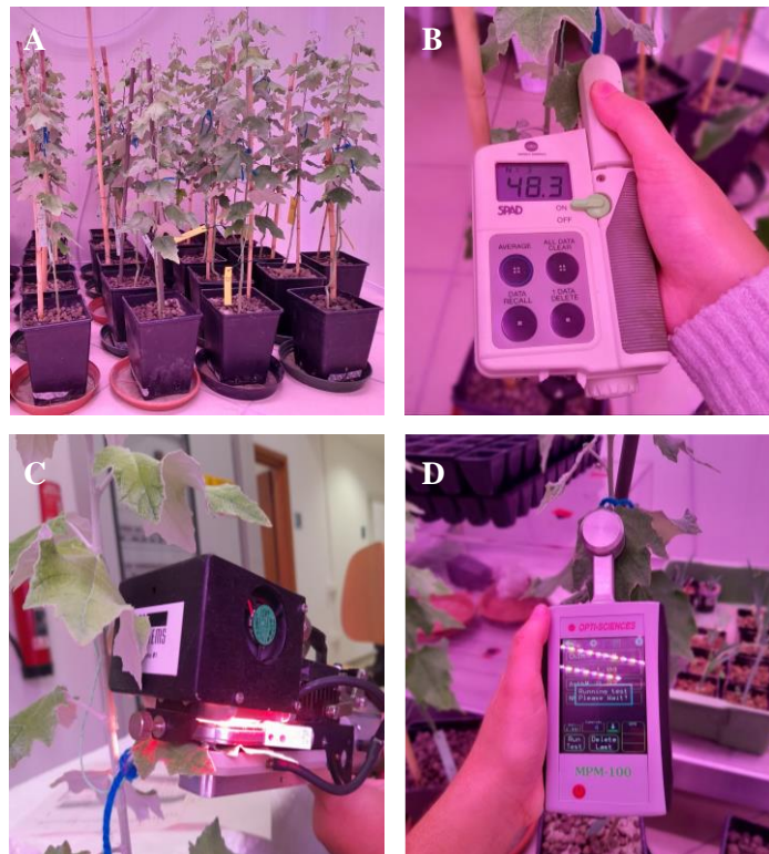
Figure 12. Non-destructive physiological measurements. (A) Populus alba L. “Villafranca” clone plants on time 0, placed in the growth chamber under controlled conditions. (B) SPAD (SPAD-502 Plus, Konica Minolta, USA) measurement on a fully expanded leaf. (C) Measurement of G_s and P_n using the portable gas exchange system, CIRAS-2 (PP Systems International, USA). (D) Flavonol measurements using the multiple wavelength pigment meter (MPM-100, Opti-Sciences, Inc., USA).
