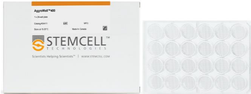
Figure 2.4 Aggrewell plate (24 wells with 1200 microwells each).
