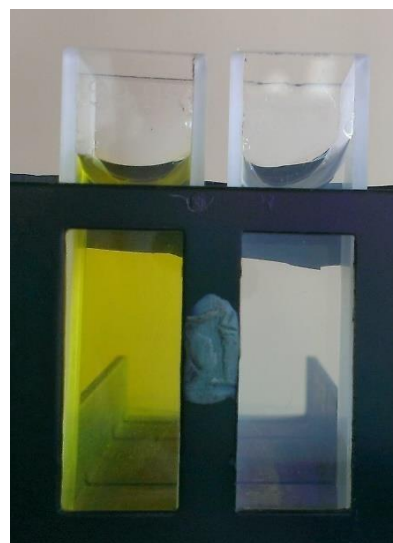
Figure 6.4. Samples in cuvettes with solutions contained CdS nanoparticles in gelatin matrix (yellow) and pure gelatin (transparent).
