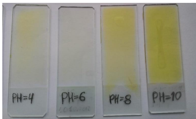
Figure 6.5. Samples of thin films of CdS nanoparticles in gelatin matrix with different pH values.
