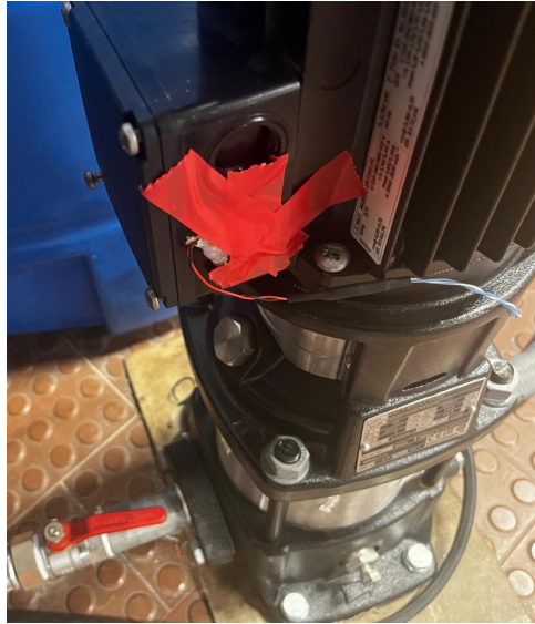
Figure 4.16: Coupling of the piezoelectric element to the pump.
