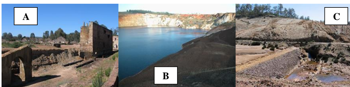
Fig 2.2- A: an abandoned building infrastructure in ruin since 1966, B- The open pit filled with AMD water and C- AMD water runoff
