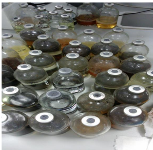
Fig 3.2- Anaerobic batch flasks used in work.
