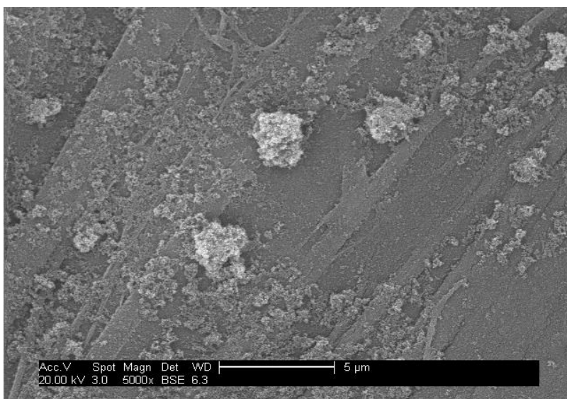
Figure 4.8 –PVDF surface after PSFD with TiO 2 (1.5 g / L at pH =1 solution) (x5000)
