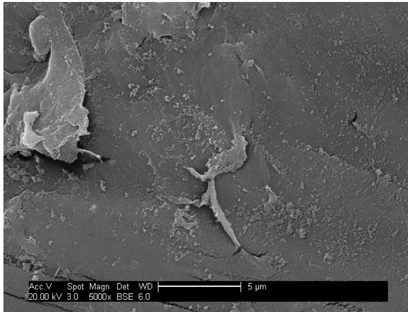
Figure 4.11 – PVDF surface after PSFD with \text{TiO}_2 (1.5 g / L at pH =7 solution) (x5000)
