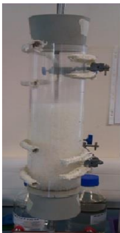
Figure 3.4 – Fixed-bed adsorption column
