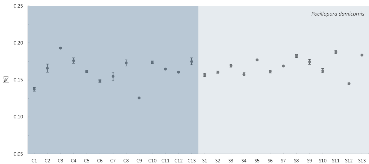
Figure A 8: average weight loss [%] between 400-440 °C for P. damicornis from control and seep sites (C1-C13: control; S1-S13: seep); average weight loss and standard deviation were calculated from three replicates per sample
