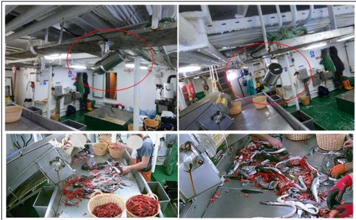
Figure 6.1: Camera installed at the sorting table (top) and images with zoom, from the integrated Electronic Monitoring and Reporting solution, the Olrac® iEMR (bottom).
