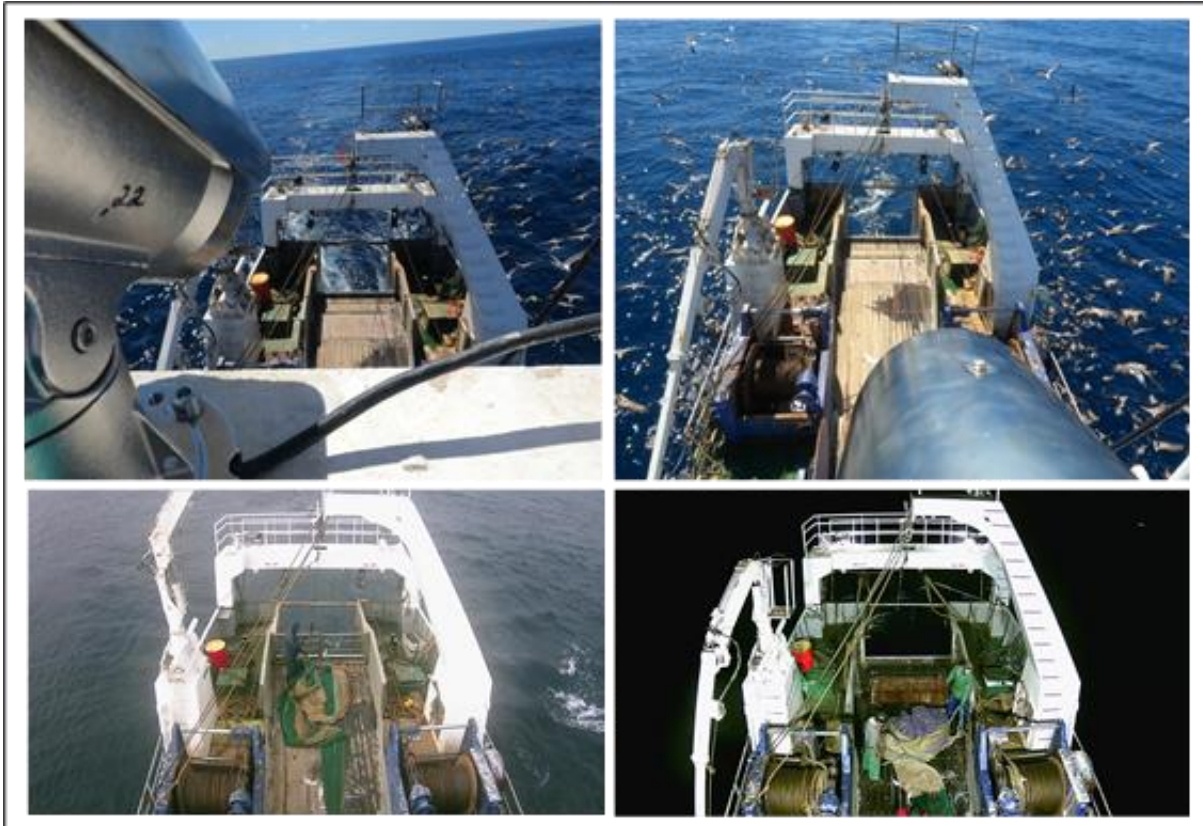
Figure 6.2: Camera aiming at the main deck (top), with its daylight (bottom left), and nightlight (bottom right) view accessed from the images of the integrated Electronic Monitoring and Reporting solution, the Olrac® iEMR.
