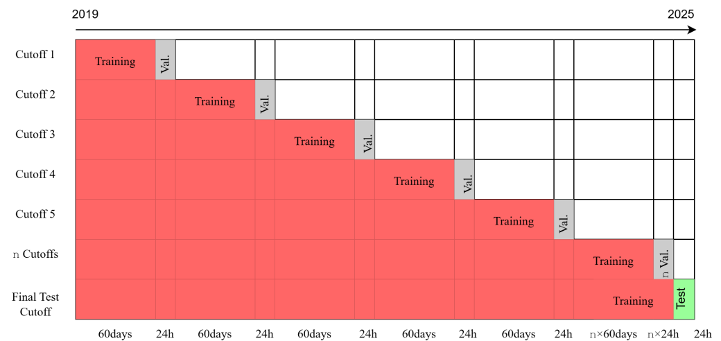
Figure 2. Phase 1: temporal validation with 33 cutoffs spaced by 60 days; each cutoff trains on all prior data and forecasts the next 24 h; the last 24 h are kept as an independent holdout.
