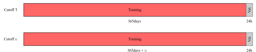
Figure 3. Phase 2: Bayesian search with four representative cutoffs and controlled training history (about 365 days at the earliest, increasing progressively); each cutoff evaluates a 24 h forecast window.
