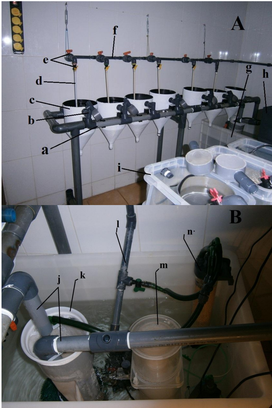
Figure 2.1: A:Schemefrom larval system of M. sculptus . a- discharging tube (outflow); b- outflow; c- tank; d- inflow pipe (6 mm); e- water flow control faucets; f- inflow tube (25 mm); g- sump; h- cubic tank i- settlement table; B: Scheme from larval system sump. j- discharging tube (outflow); k- 50 µm filter bag; l- inflow; m- skimmer; n- sand filter.
