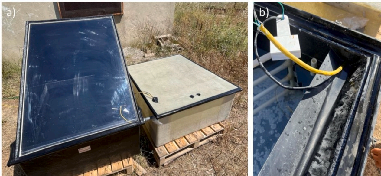
Fig. 3. (a) Prototype 1 solar still unit, with temperature and conductivity sensors, and the reservoir for desalinated water storage; (b) detail of the gutter placed inside of the solar still for desalinated water collection.
