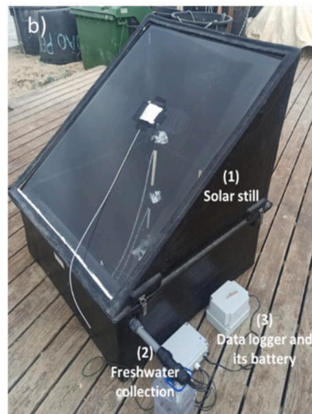
Fig. 4. (a) Prototype 1 design with dimensions; (b) Prototype 1 (1) with the pipe for freshwater collection (2) and the data logger (3).
