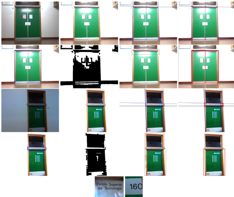
Fig. 3. Top row, from left: input image, brightened and sharpened image, detected horizontal and vertical edges, and intersection points. Second row: detected rectangles of method (1), plus segmented image, detected rectangles and selected ones of method (2). Third and fourth rows: another door. Bottom row: examples of texts extracted from doors.
