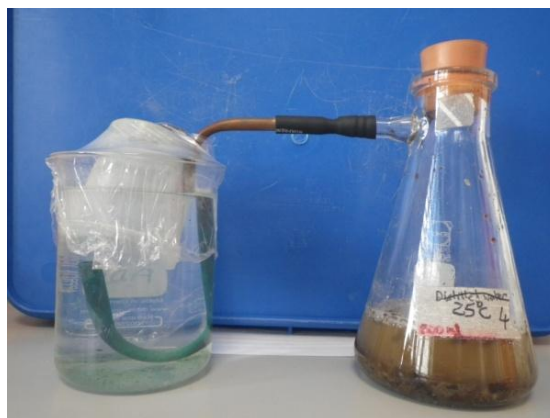
Figure 5 Bioreactor system: conical flask fermenter with the gas collector on side-arm.
